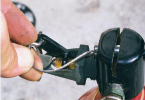
The hook isn't actually attached to the little arm, just run through the little hole in it. It gets pulled straight back when pulled and the arm does its thing. You should be able to gently push the cable forward (only about one half inch total) with your right hand and back the hook-end
